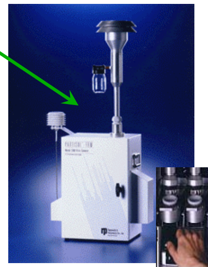
Partisol-FRM Model 2020-D Dichotomous Low Volume Single Event Air Sampler
